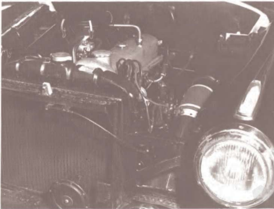
The overhead-camshaft six-cylinder engine installed in the 220a being assessed by Rover. Maximum output of 85bhp was achieved at 4,800rpm.
