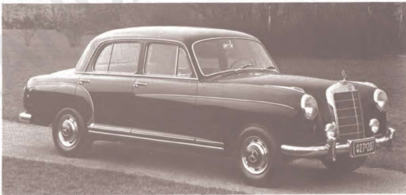
The 220S saloon is immediately identifiable from its 220a counterpart by the use of additional chrome to emphasize the double curve of the front wings.
