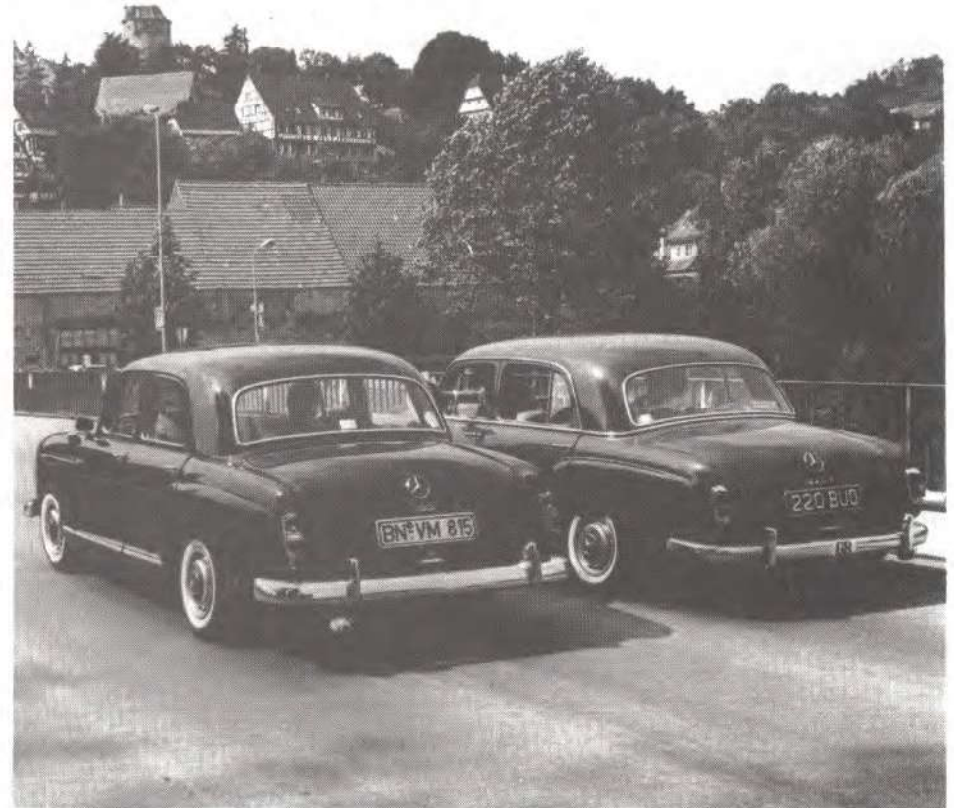
An interesting picture by Colin Peck showing the post-1957 rear lamps on a 180c alongside the pre-1957 type on a 220S. By the time the 180c was built the four-cylinder Pontons had inherited the larger rear windows originally confined to the six-cylinder models.
