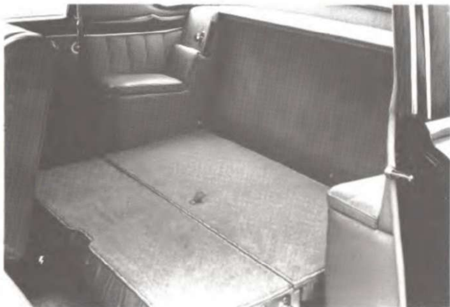
A sensible design feature of this 220S coupe is the fold-flat rear seat, which offers substantially more luggage accommodation when only two people are being carried.
