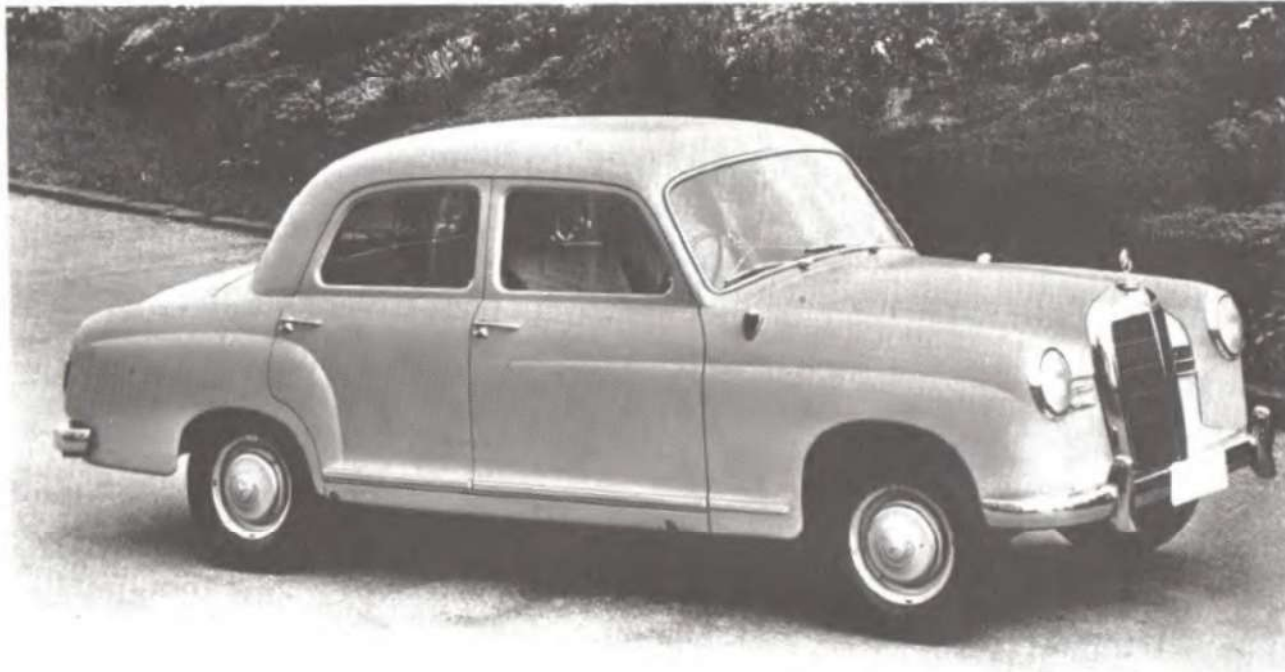
One of the first 180 saloons to be supplied with right-hand drive. From 1954 the 180 was also offered in diesel-engined form as the 180D, and although the engine was almost identical to that previously fitted to the 170S-D, the lighter weight of the newer car meant that higher gearing could be used.
