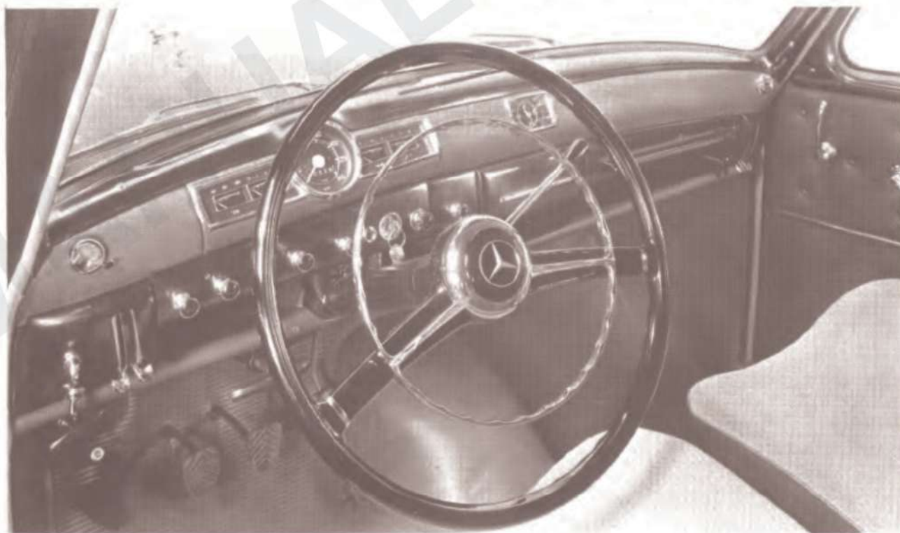
The front compartment of the 180 on its announcement in 1953. A large-diameter steering wheel has been a characteristic of Mercedes-Benz cars for many years.
