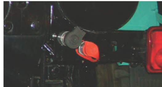
Plug connections at rear [H50] on the right in direction of travel: delivery line (red) and return line (black)
