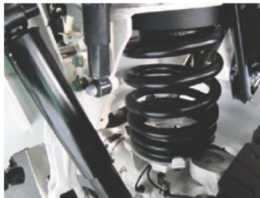
Coil springs with telescopic shock absorbers
