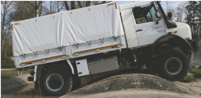
Driving over sharp crests possible thanks to large ramp breakover angle and angle of approach/departure
