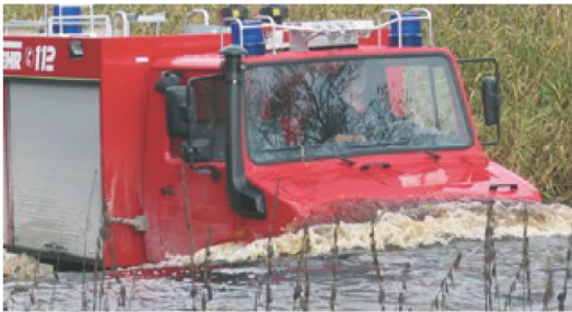
Special equipment, special parts for fording capability to 120 cm [Z16]
