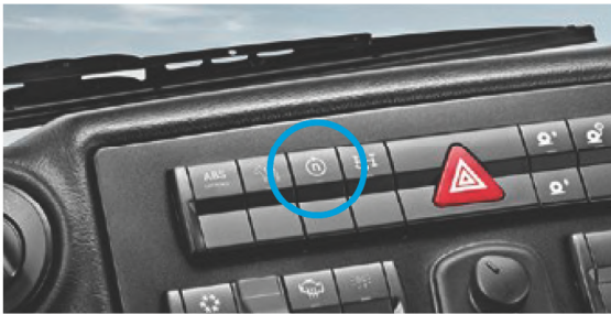
Switch to select engine control characteristic on dashboard (middle)
