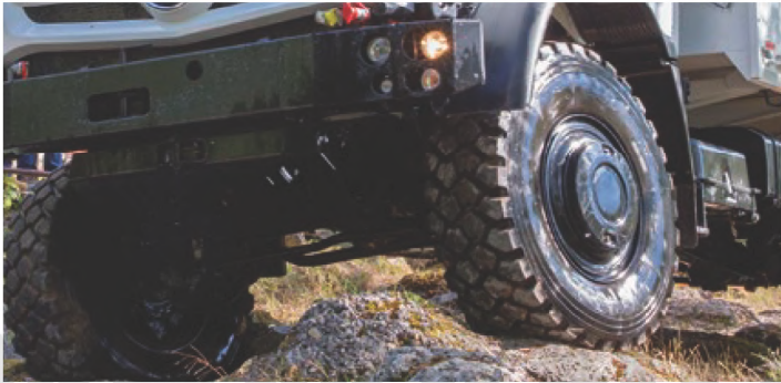
Driving over obstacles optimised by asymmetric arrangement of the axle differentials
