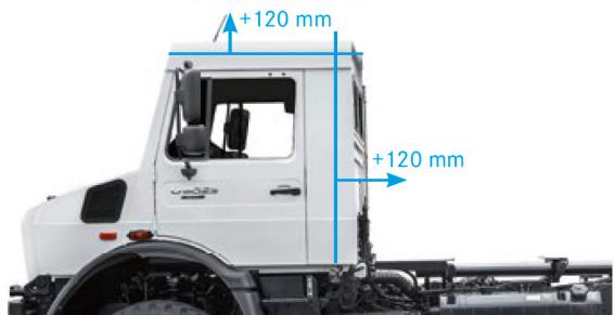
Proven cab-behind-engine with greater volume than the predecessor model
