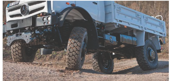
3-point mounting of engine, gearbox and cab. Double 3-point body mounting
