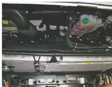
Coolers for charge air and engine cooling water arranged next to one another
