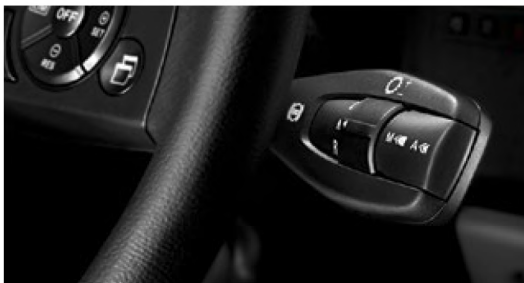
Multifunction lever and multifunction keys on the steering wheel
