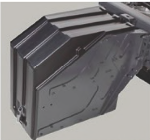
[C7K] Battery support, batteries above each other
