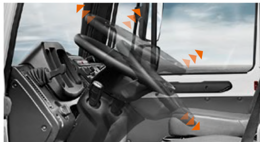
Adjustment range of the steering column
