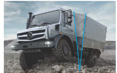
Diagonal torsional flexibility with torque tube technology
