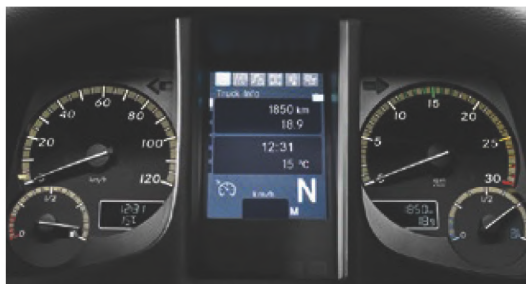
Gear selection indicator in instrument cluster
