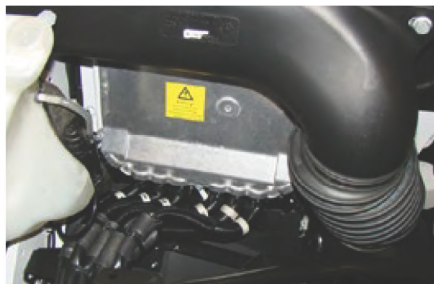
Central plug connections in the engine compartment
