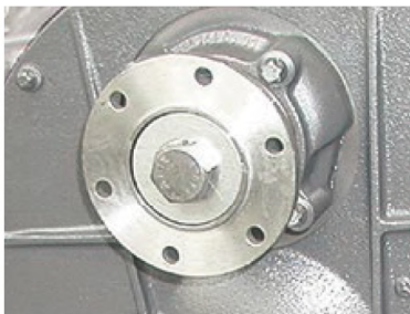
[N19] Transmission PTO, very high-speed, with flange
