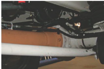
Torque tube protects propeller shaft from soiling and damage, even in extreme terrain
